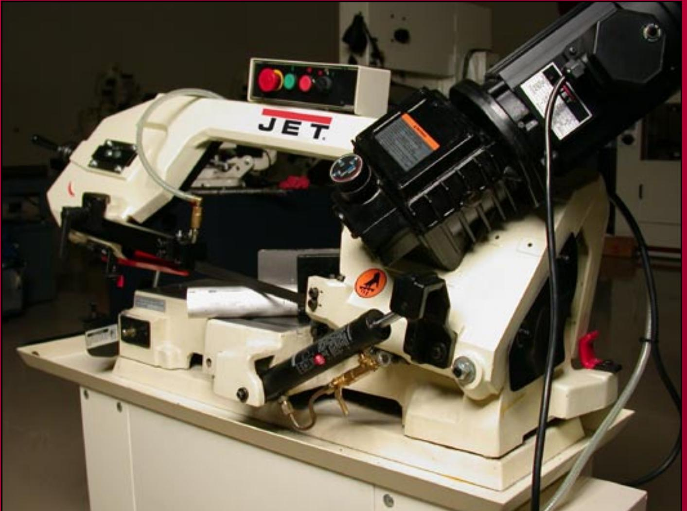
The new JET® HBS814GH horizontal bandsaw features a heavy duty gear drive to provide accurate and vibration free cutting. Featuring an 8" vertical cutting capacity, hydraulic downfeed, and enclosed coolant system. Powered by a 1 horsepower motor rated at 1720 RPM it provides three blades speeds: 135, 197, 256 SFPM. Changing blade speeds is fast and easy with the turn of a dial, no belts or pulleys to replace. Mitering or straight cut-off is no problem for the HBS-814GH.
