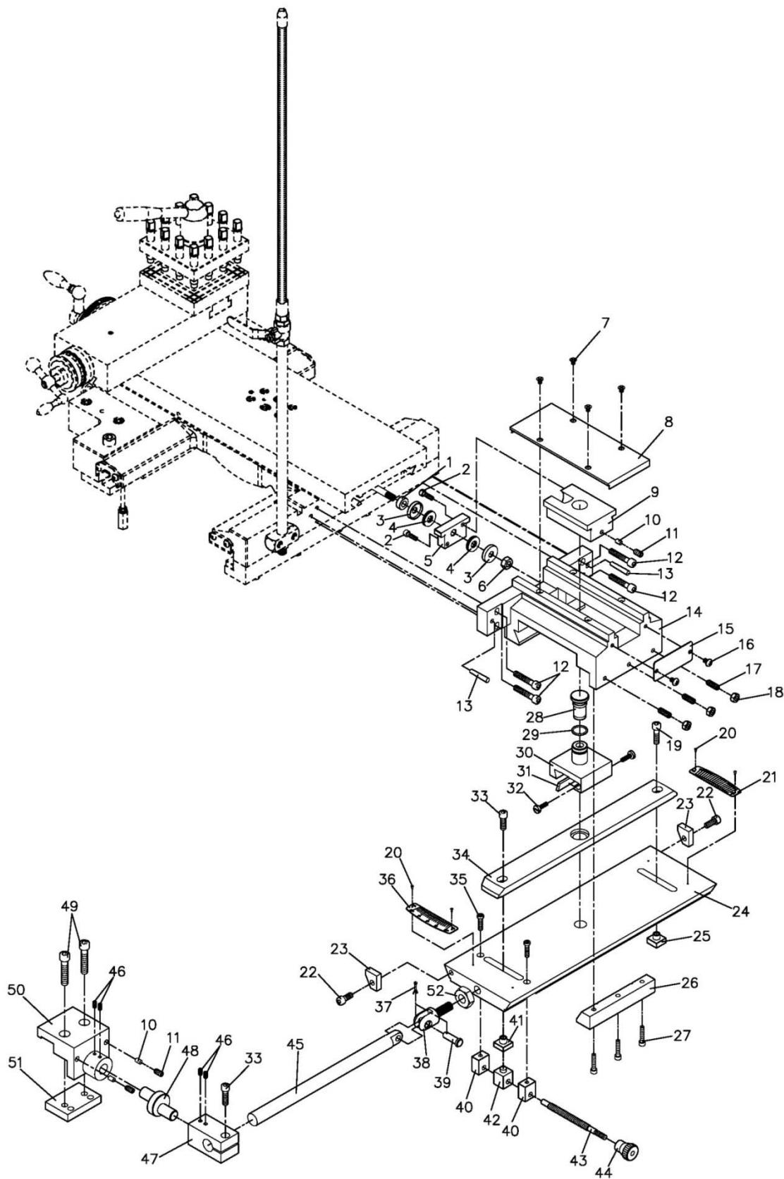
**Taper Attachment Assembly for EGH-1740, 1760 JET® ELITE Lathes**
