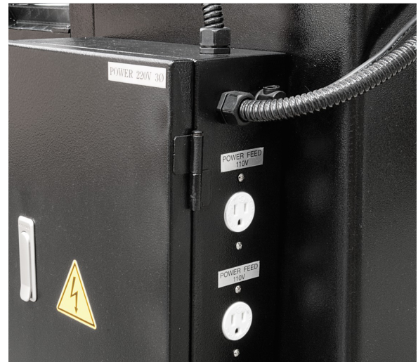
ELITE MILLS FEATURE TWO CONVENIENT PLUG-INS FOR POWERED ACCESSORIES
